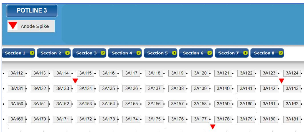
Figure 8. Spike alert in pot control system.
